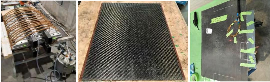
**Figure 4.** RTM tooling to manufacture composite plates (left), basic composite plate (centre) and composite plate with sensors (right).
