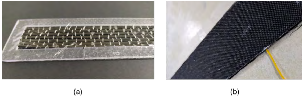
Figure 1. Manufacturing process of specimens with integrated OF a) Resin 3D printed spacer with grooves to extract the OF, b) specimen with an integrated fiber optic sensor.
