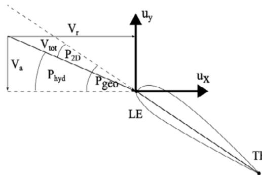
**Figure 5.** Definition of 2D profiles blade pitches.
