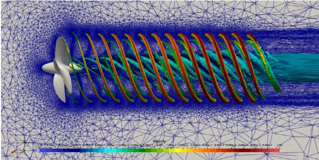
**Figure 1.** Flow structure and adaptive mesh visualization.
