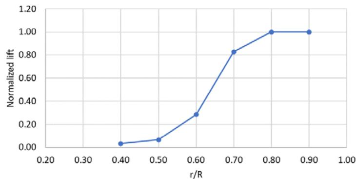
**Figure 6.** Importance of lift at different radius of the blade.
