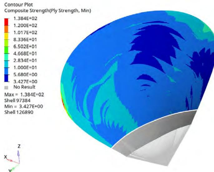
**Figure 11.** Minimum safety factors SF\_CSiapp calculated in each ply
