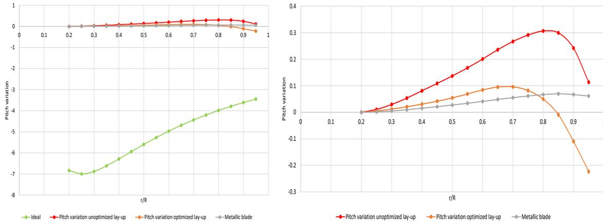
**Figure 10.** Comparison of the pitch variation for different material: with ideal pitch (left) without (right)
