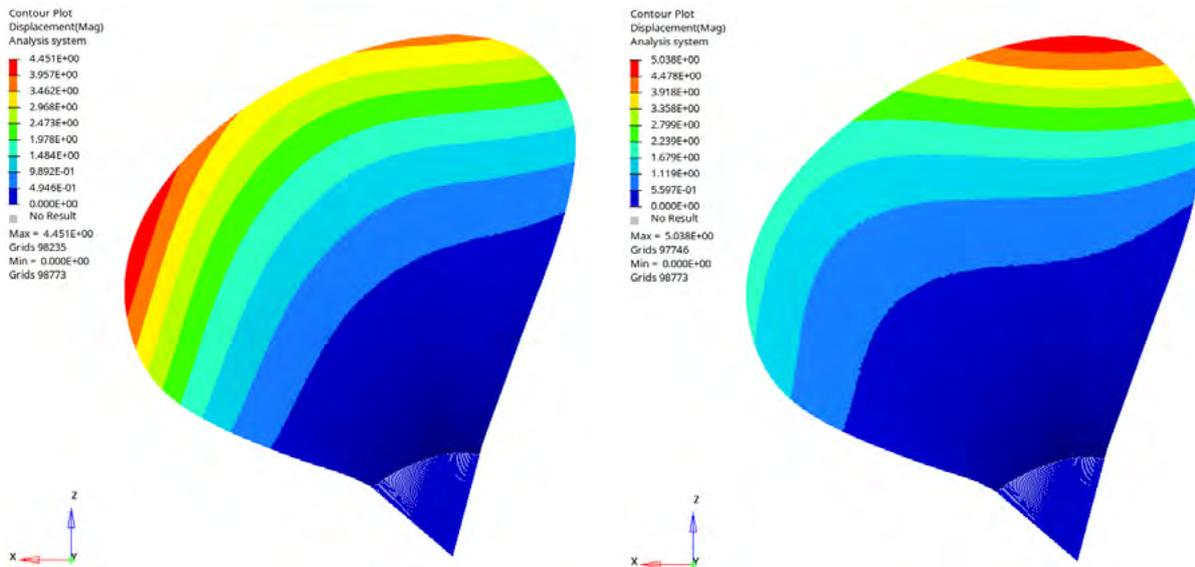
Figure 9. Variation of displacement between reference shape ( $J = 0.88$ ) and the design shape ( $J = 0.69$ ) with unoptimized (left) and optimized stacking (right).
