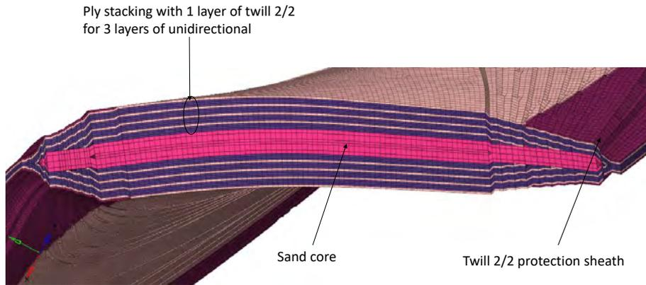
Figure 8. Cross sectional view and stacking of the FEM model.
