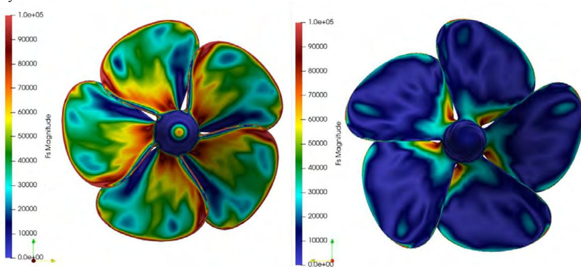
Figure 4. Total surface force applied on the full scale propeller at  $J=0.88$  (sea margin 30).
