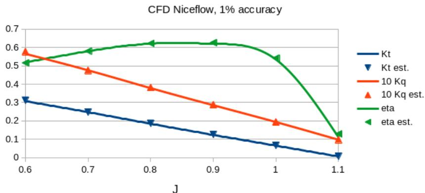
**Figure 2.** Adimensional coefficients of Le Palais propeller.
