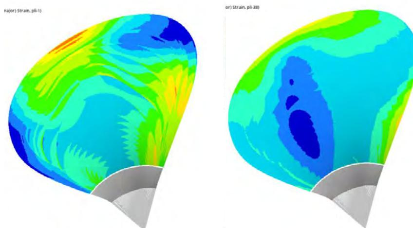
**Table 12.** Strain field on the blade: extrados (left) and intrados (right).
